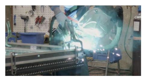
CUT PROFILES AND WELD TOGETHER
