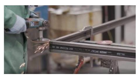
GRIND WELDS TO FLUSH SEAMLESS SURFACE
